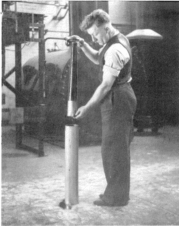
Fig. 3—Withdrawing a 25-inch Cone from its Packing Tin in which it is immersed in Compound. Note how the Cone is attached to the Lid of the Tin.
