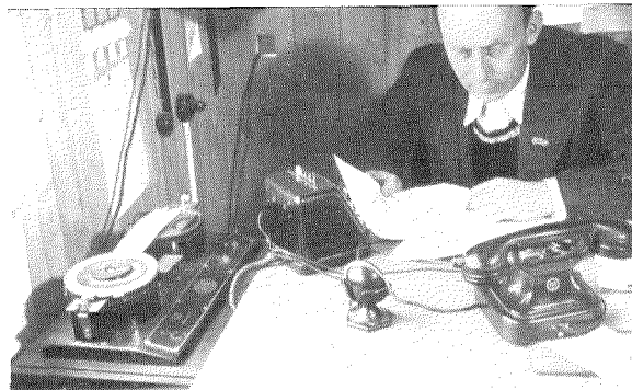
Lorenz Steel-tone Wire Machine ("Textophone") installed in the Office of the Director of the Organization Committee in Garmisch-Partenkirchen (Control Station).
