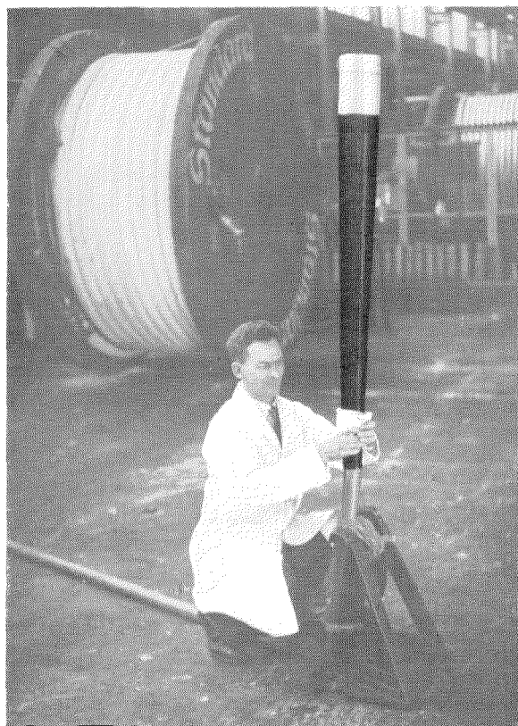
Fig. 1—Mounting a 50-inch Cone on a Cable End. The Cone should be adjusted by gripping with Rag near its Base as shown, and should not be pressed down from the Top.
