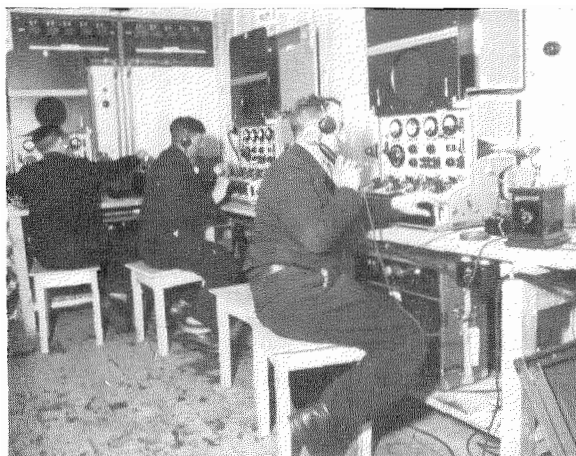
Olympic Transmitter at Garmisch-Partenkirchen with the Lorenz Speech Input Amplifier (V35).
